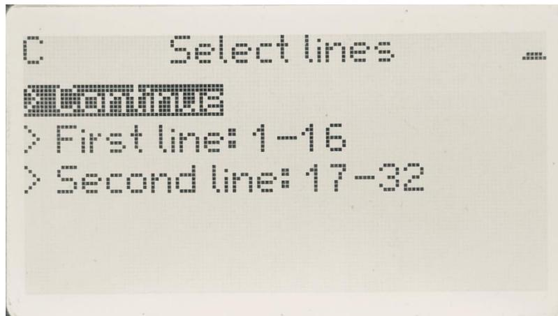
**FIGURE 24 - SELECTION OF THE ORDER OF THE ELECTRODES**
