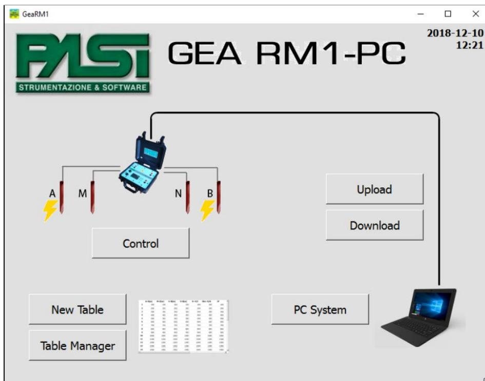
FIGURE 2 - CONNECT THE INSTRUMENT TO THE PC AND RUN THE SOFTWARE. CLICK ON "NEW TABLE" TO CREATE A NEW TABLE
