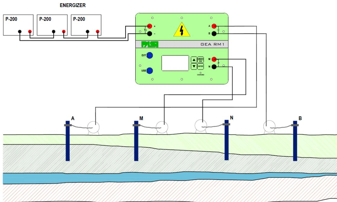
**FIGURE 1 - HARDWARE CONNECTIONS**
