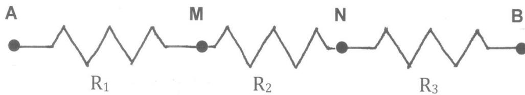
$$R_1 = R_3 = 470 \, \Omega \quad (5 \, \text{W})$$
