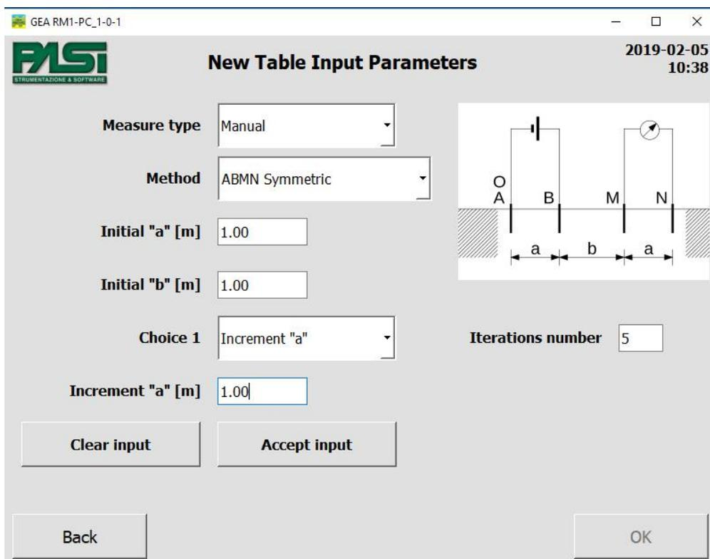
**FIGURE 40 - PAGE CREATION NEW MANUAL TABLE WITH DIPOLO-DIPOLO**
