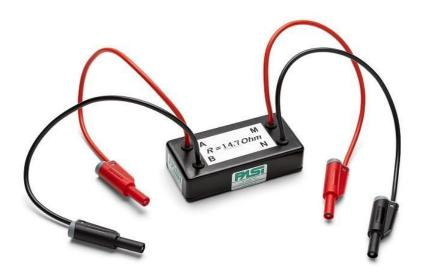
Performing the measurement (after connecting of A, B, M, N to the respective connectors on the resistivity meter and after connecting the energizer to the earth resistivity meter),  $\Delta V/I$  ratio must be equal to the value of R2 = 15  $\Omega \pm 10\%$ .
