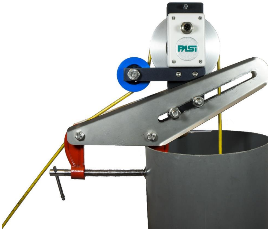
FIGURE 1 - ENCODER PROPERLY INSTALLED
