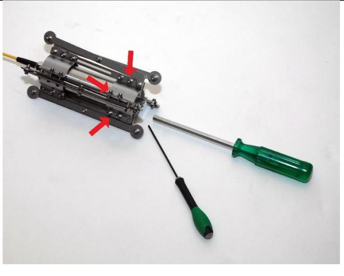
The centering device is shown with three red arrows pointing to specific bolts. A green-handled screwdriver and a black-handled screwdriver are placed next to it, indicating the tools used for tightening. |
