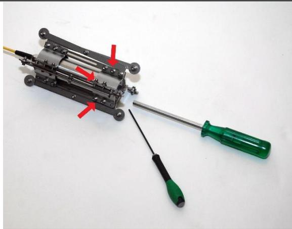
5) The diameter of the centering device can be adjusted as indicated by sliding the two flanges along the device
