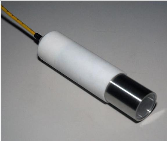
The camera head is inserted into a white cylindrical Teflon shield.                                              |
