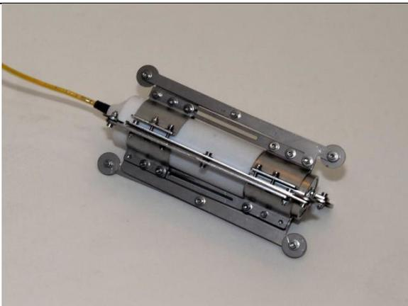
The camera head assembly is mounted inside a complex metal centering device with rollers and adjustment screws. |
