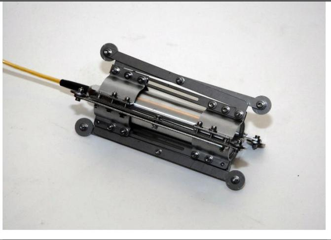
The Well-Camera head is inserted into the narrowest part of a complex, metallic centering device. The device has several adjustment bolts and a curved top section.                                           |
