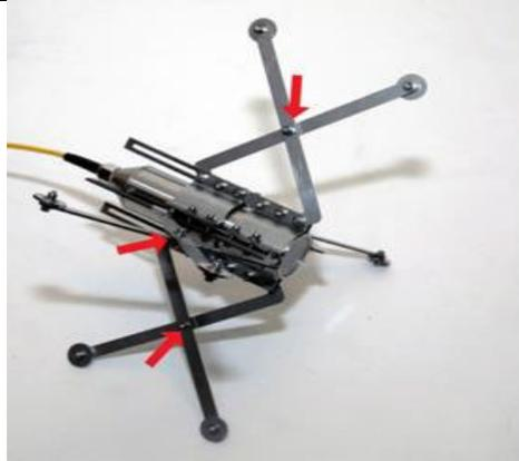
7) Fix the ASPO fiber glass cable to the teflon shield as shown in the picture.
