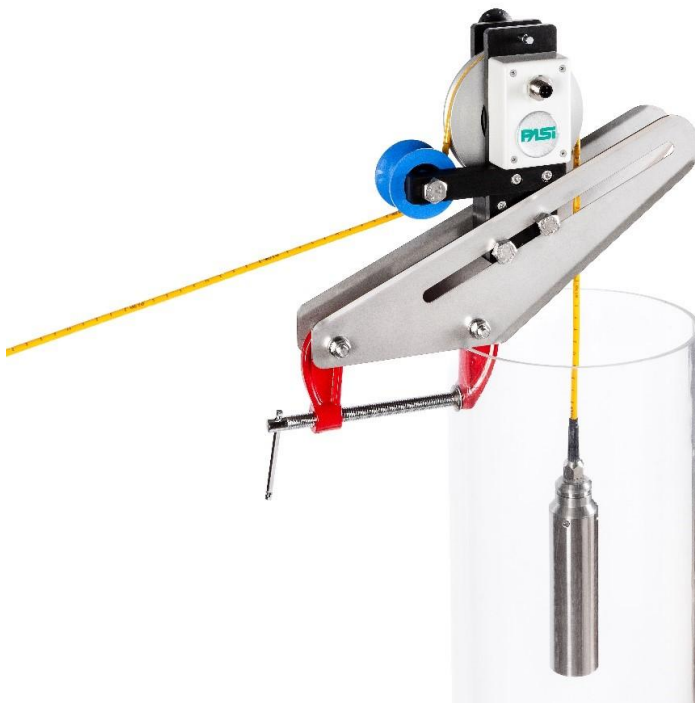
FIGURE 9 - ENCODER PROPERLY INSTALLED
